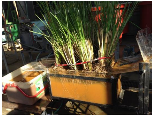
Figure 3. Set-up System 3: 4 rows vetiver, 100 g silt circulated
